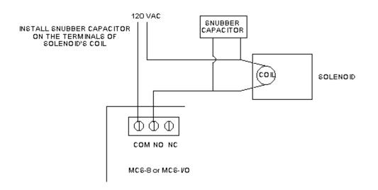
3. Install a Snubber capacitor across any coil that has an inline series switch or contact with our relay output.
